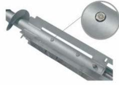
Air Flow through the rotating shaft to clean the mesh area of Roto sifter basket.
