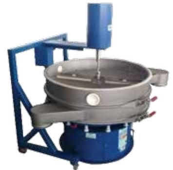
Rotary brush operates independently with the Sifter. Lumps are broken apart & cleaned by horizontal scraping motion.
