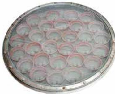
Mesh De-Blinding Kit is placed below the mesh. elastomer or polyme Balls tap the screen to avoid blinding.
