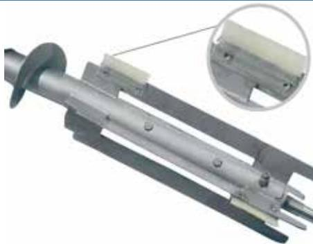
The brush cleaning system. Clean the Roto Sifter basket with the help of brush attached to the rotary shaft.
