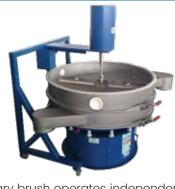
Rotary brush operates independently with the Sifter. Lumps are broken apart & cleaned by horizontal scraping
