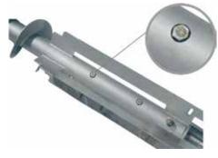
Air Flow through the rotating shaft to clean the mesh area of Roto sifter basket.
