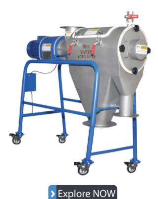
SIVTEK Roto Sifter is designed to meet high-capacity scalping and sifting for both large and small process applications. It is ideal for handling a wide variety of powder, granules and other free-flowing materials.
